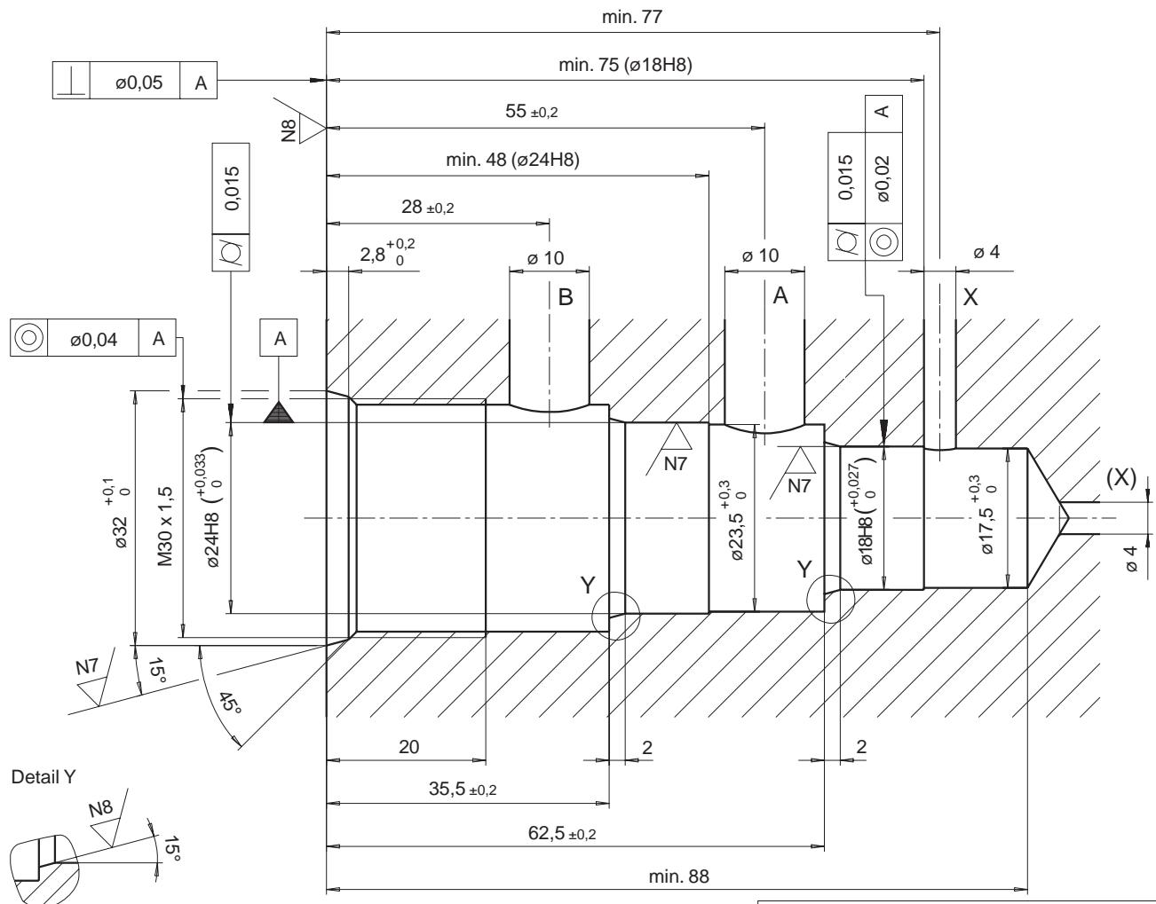
Bores A, B and X can be positioned anywhere around circumference.
