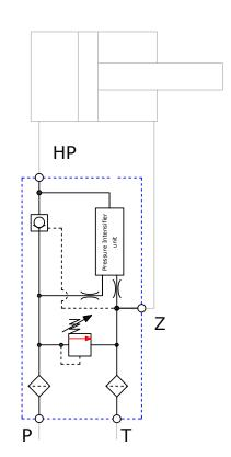
Inlet flow: Min. 2 LPM to max. 20 LPM
