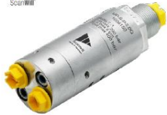
MP-S: In-Line mounting Pin: 15 - 207 bar Pout : 30 - 800 bar Qin max.: 8 LPM
