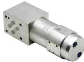
MP-C: CETOP/NG6 mounting Pin: 15 - 207 bar Pout: 30 - 500 bar Qin max.: 15 LPM
